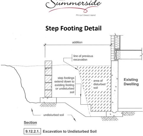
Example: Typical footing to connect a new frost wall to an existing full-depth foundation wall
