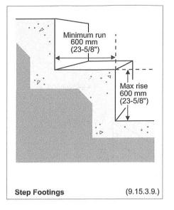
Per Section 9.15.3.9 of the NBC, the vertical rise of a step footing is limited to a <u>maximum</u> of 600mm and the horizontal run is required to be a <u>minimum</u> of 600mm. Maintain the thickness of the strip footing throughout the rise and run of the step footing.
